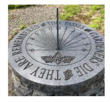
A sundial contains a gnomon, or a thin rod, that casts a shadow onto a platform etched with different times. As the sun changes relative positions over the course of a day, the rod's shadows change as well, showing the change in time.
